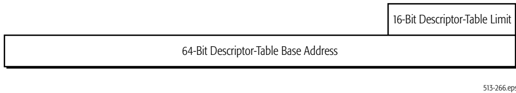
Figure 4-8. GDTR and IDTR Format—Long Mode
