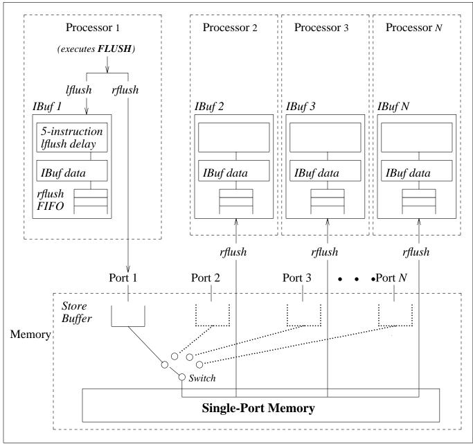
The IBuf of each processor consists of three elements: a 5-instruction local flush (*lflush*) delay that delays the execution of locally generated FLUSHes by at most 5 instructions; the IBuf data; and a remote flush (*rflush*) FIFO that contains flushes generated by remote processors. Processor 1 executes a FLUSH A by issuing a local flush (*lflush*) command to its IBuf and placing a remote flush
