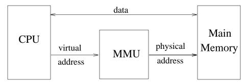
The MMU translates virtual addresses from the CPU into physical addresses, as shown above in Figure H-1. A 32-bit virtual address is translated to a 36-bit physical address, providing for a 64-gigabyte physical address space to support large physical memories and memory mapping of 32-bit busses (for example, VME or MultiBus II). A physical address is logically composed of an offset into a 4K-byte page and a Physical Page Number as follows:
