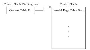
At any one time only one address space is active. The current active address space is identified by its context number. This provides the offset into the Context Table used to retrieve the pointer to the Level-1 Page Table for the address space.
