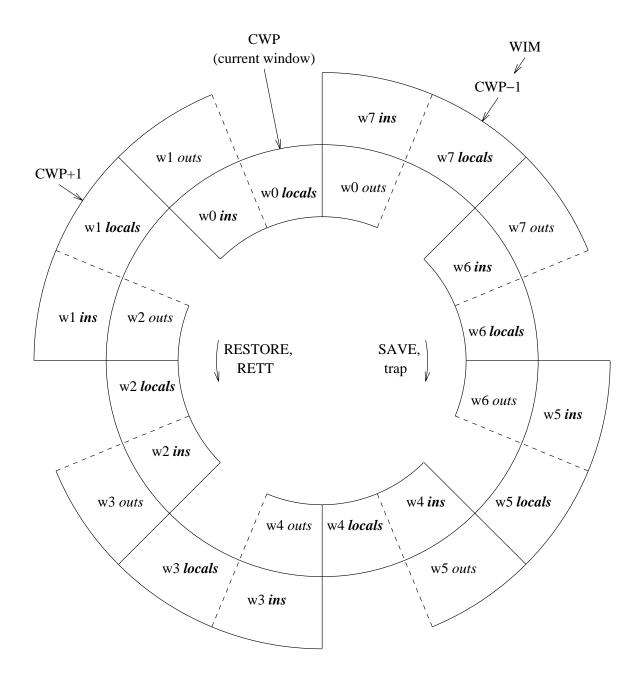
Figure 4-2 The Windowed r Registers
