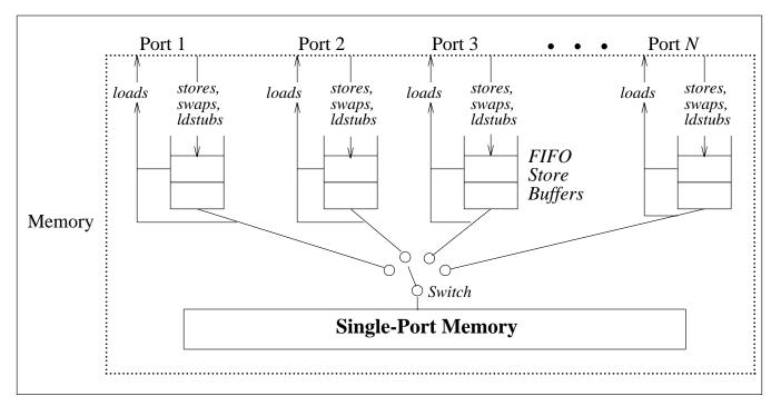
Stores, FLUSHes, and atomic load-stores issued by a processor are placed in its dedicated Store Buffer, which is FIFO. Thus the order in which memory executes these operations for a given processor is the same as the order in which the processor issued them. The memory order of these operations corresponds to the order in which the switch is thrown from one port to another.
