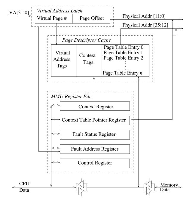
Figure H-5 Block Diagram of Reference MMU
