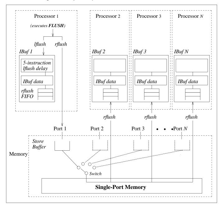
Figure K-3 Operation of the FLUSH Instruction
