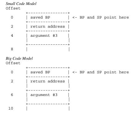
As the above diagrams show, the third argument is at offset 4 from register BP in a small code model and offset 6 in a big code model.
