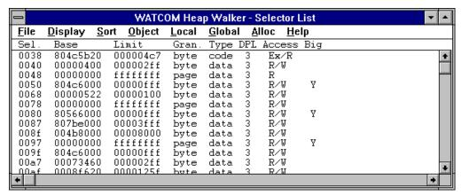
Figure 136. The Selector List displays all valid ring three selectors.
