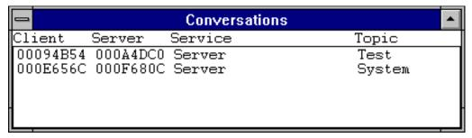
Figure 174. The Conversations window tracks all conversations currently active in the system.
