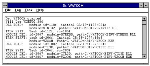
Figure 178. The Dr. Watcom window contains the event list which records and displays events occurring under Windows.
